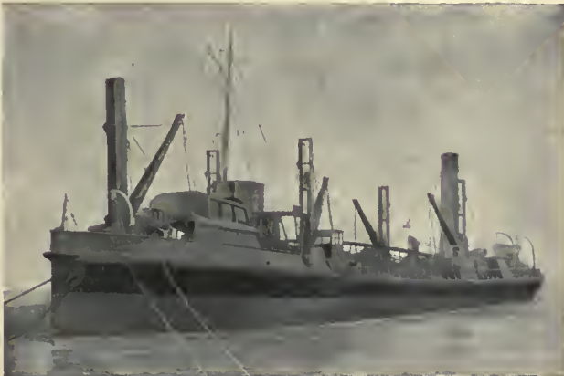
FIG. 9.—Twin-screw grab-dredger, "Miles K. Burton," built for the Mersey Docks and Harbour Board by Wm. Simons & Co.
